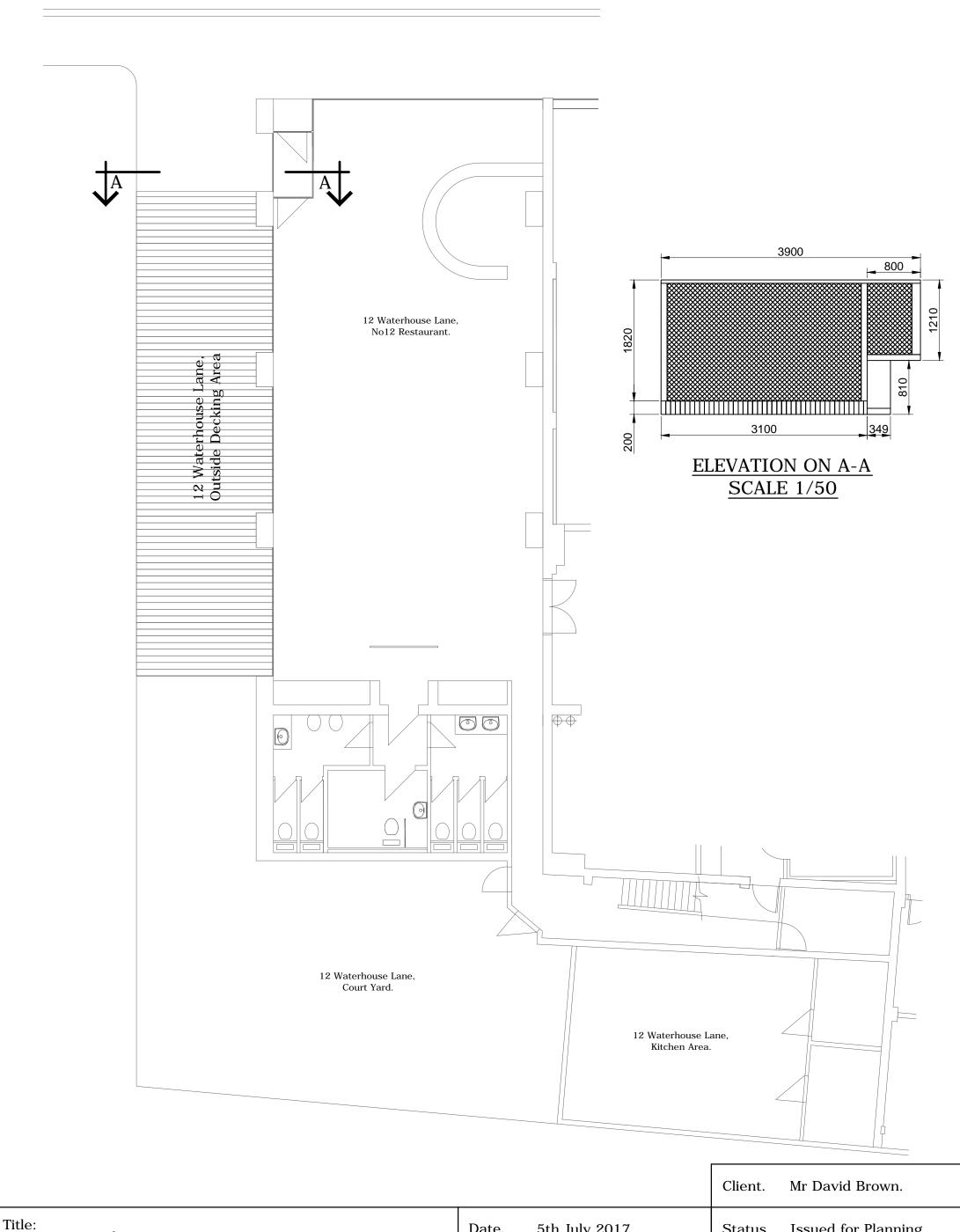
12 Waterhouse Lane, Existing Ground Floor Plan showing New Outdoor Seating Area
